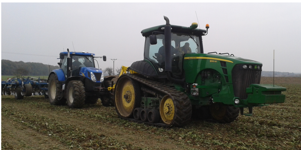
Fig. 2. Testing set. From the right: track tractor JD 8320 T, special tool for measurement of draught force and tractor NH 7050 pulling cultivator with tines
